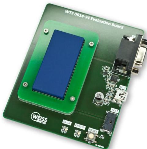
The Evaluation Board is powered via USB, so you need to connect it either to a spare USB port on your PC or you may use a USB wall power adapter.
